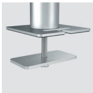
Bolt-through fixing for desk thicknesses from 14 to 44 mm and desk hole diameters from 60 to 80 mm
